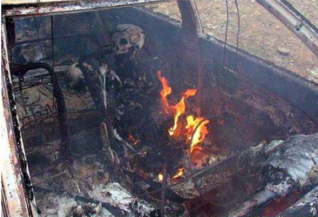
PHOTOGRAPH 5: Fat absorbed by porous material burning in a limited area (Wick Principle). From: J. DeHaan and E. Pope, Combustion Properties of Human and Large Animal Remains [35]
